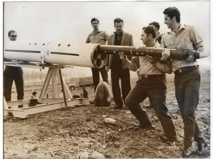
The sole high-quality picture of BST-1. The is rocket inserted to the launch canister 6
